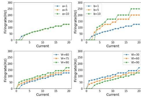
Figure 3. The response curve (the f-I curve) of the IQIF neurons. Top-left: the curve is relatively insensitive to the parameter  $a$ . Top-right: The gain, or the slope of the response curve, of the IQIF neuron can be changed by the parameter  $b$ . Bottom-left: the resting potential  $V_r$  does not affect the gain but can change the rheobase of the response curve. Bottom-right: the spike threshold  $V_i$  has an effect on the response curve similar to  $V_r$ .
