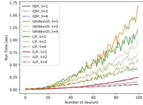
Figure 5. Run time of IQIF and other neuron models as a function of the number of neurons in an all-to-all network. The tests were performed with single thread ( $t=1$ ), two threads ( $t=2$ ) and four threads ( $t=4$ ). The IQIF is faster than Izhikevich and LIF models and is comparable to quantized LIF (ILIF) in all conditions.
