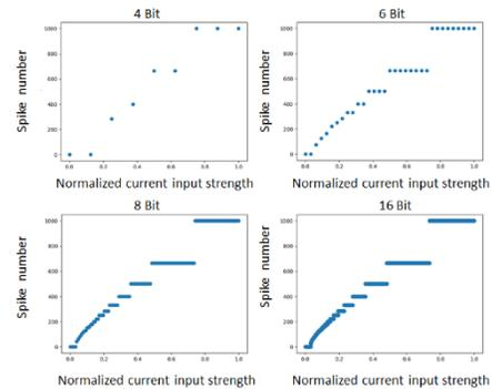
Figure 6. The response curve of the IQIF neurons with different integer bits. The IQIF neurons work well with integers of 8-bit or larger with a firing rate below 300 Hz
