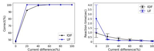
Figure 8. The psychometric functions of the decision task performed by decision networks made of IQIF or LIF neurons. Top: Accuracy (percentage of correct) as a function of the difference between the input currents. Bottom: Reaction time as a function of the difference between the input currents. IQIF neurons perform comparably with the LIF neurons
