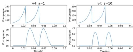
Figure 2. The membrane potential of a postsynaptic IQIF neuron (bottom) in response to the presynaptic input (top) for different values of the parameter  $a$  (left versus right). The membrane potential relaxes back to the resting state faster if  $a$  is larger.
