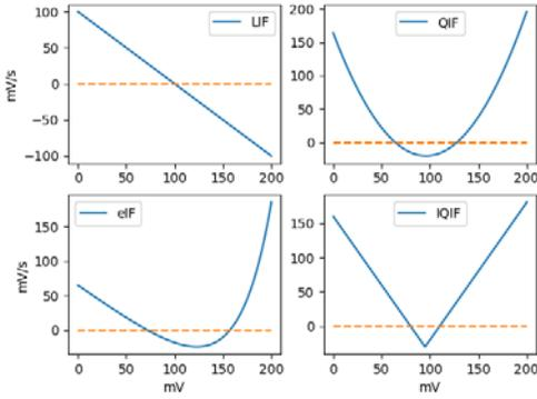
Figure 1. The  $dV/dt$  vs.  $V$  plots for four neuron models: LIF, QIF, EIF and IQIF. The intersections of the curve and the  $y = 0$  line represent the equilibrium points of the models and the sign of the slope at each intersection indicate its stability. The LIF model has only one stable equilibrium point presenting the resting state, while the other three models have two equilibrium points with one stable and one unstable which represents the spike threshold.
