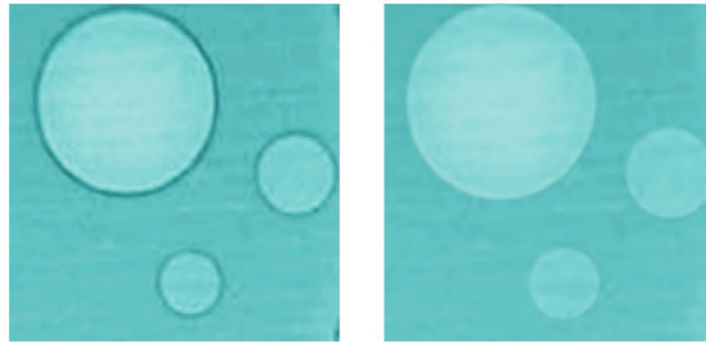
Fig. 4. X-ray image obtained with phase contrast (left) compared (right) to the corresponding (simulated) absorption radiograph.
